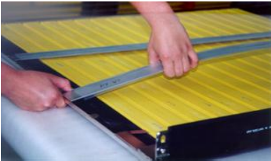
Figure 13 - Maintenance / Nettoyage du contact I
